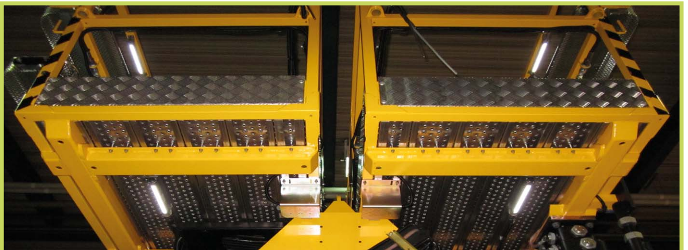
AmbitLED - Lighting on the work basket
