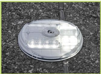
The MarkLED EXIT combines two tunnel safety lighting systems. It is a combination of guidance and escape route light, and the road studs (optical guidance system) are typically installed at distances of 12.5 m and 25 m respectively. The MarkLED EXIT is therefore equipped with two separate lighting areas with two different characteristics, usually installed at a distance of 25 m, using the same connection system, which in combination makes the system very economical.
