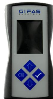
Programming device with menu guide for set-up, programming and status recognition of the control unit. Communication with the control unit occurs through radio.
