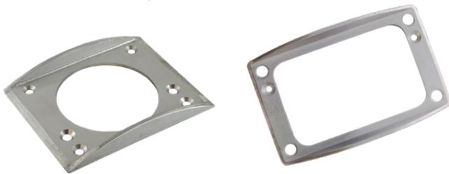
In winter, there is often the problem that the snowploughs touch the signal units when entering and exiting the tunnels. That entails that the MarkLED can be sheered off and should be exchanged. Against it we can offer a protective plate. That protects the first MarkLED's at the entrance and exit of the tunnels.
