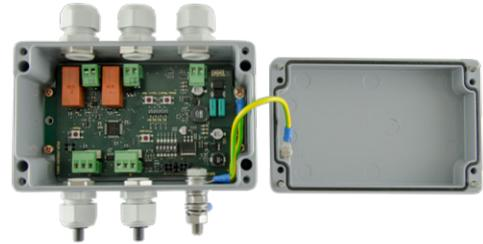
The cold conductor monitoring is used for detecting defective installations or lights that are not connected. The monitoring is automatically activated as soon as the lights are switched off.
