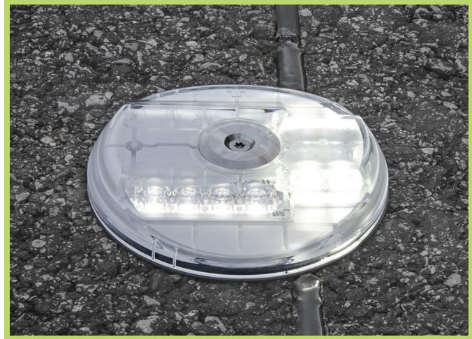
The MarkLED EXIT combines two tunnel safety lighting systems. It is a combination of guidance and escape route light, and the road studs (optical guidance system) are typically installed at distances of 12.5m and 25m respectively. The MarkLED EXIT is therefore equipped with two separate lighting areas with two different characteristics, usually installed at a distance of 25m, using the same connection system, which in combination makes the system very economical.
