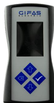
Programming device with menu guide for set-up, programming and status recognition of the control unit. Communication with the control unit occurs through radio.
