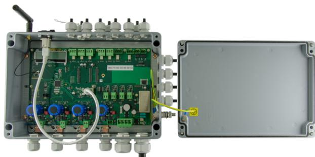
The control unit for all GIFAS systems is designed for 4 output lines. Each channel can be loaded with up to 10 A.
