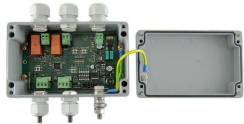
The cold conductor monitoring is used for detecting defective installations or lights that are not connected. The monitoring is automatically activated as soon as the lights are switched off.
