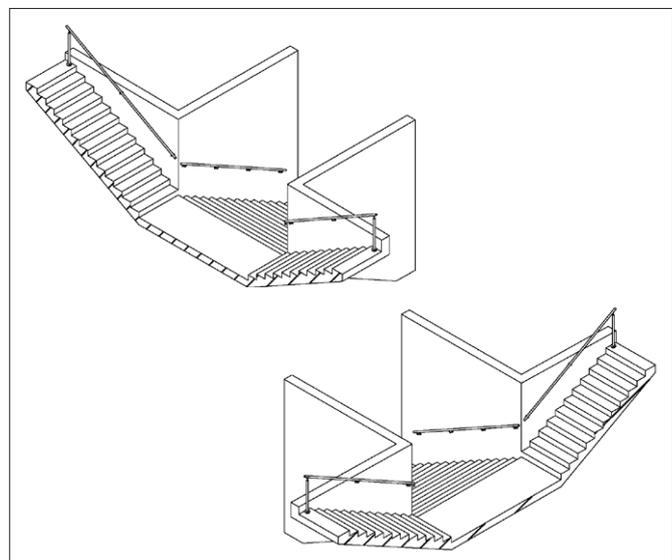
3D drawing of LaneLED INOX42 handrail
